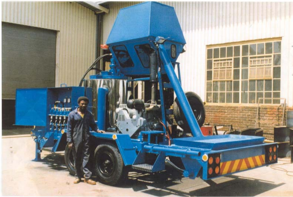
Photograph 1 Mobile Bitumen Rubber Blender
