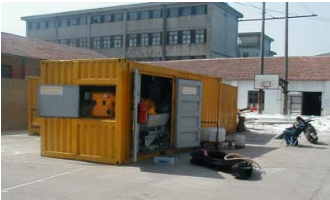
Photograph 2 Containerised Bitumen Rubber Blender used in China
