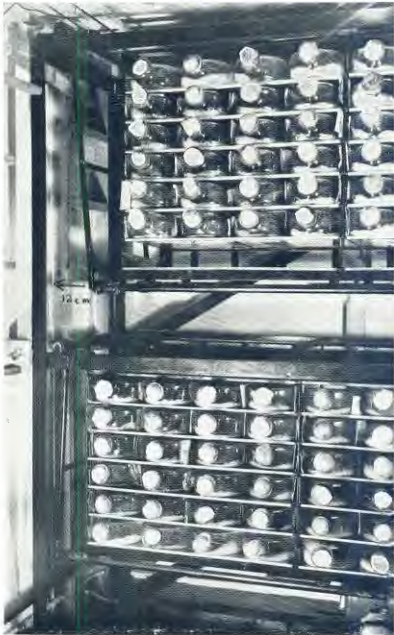
FIG. 1.—Apparatus for agitating liquid Strain 19 culture in shake flasks by reciprocating movement.
