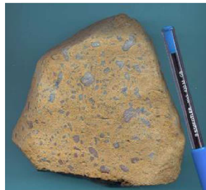
Figure 20. Altered macrocrystic olivines in highly altered clay matrix of one of the Makongonio meta-kimberlites (photo Bhebhe).
