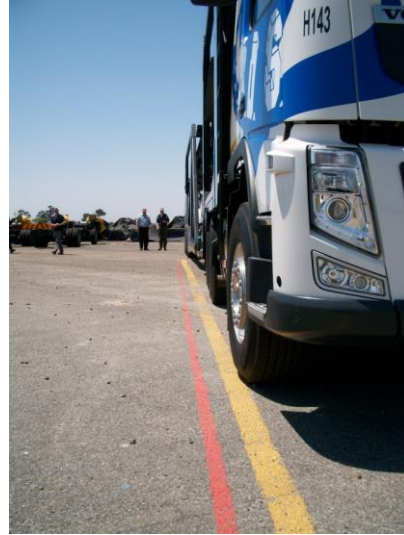
Figure 3: The modified Unipower Maxiporter undergoing low-speed turn testing
