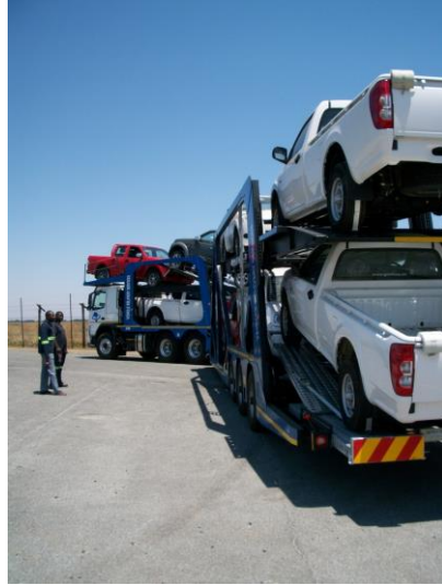
Figure 3: The modified Unipower Maxiporter undergoing low-speed turn testing
