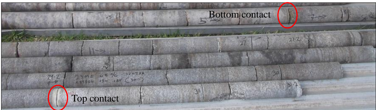
Figure 8.10: Photograph indicating the condition of the top and bottom contacts of the Bastard Merensky Reef.
