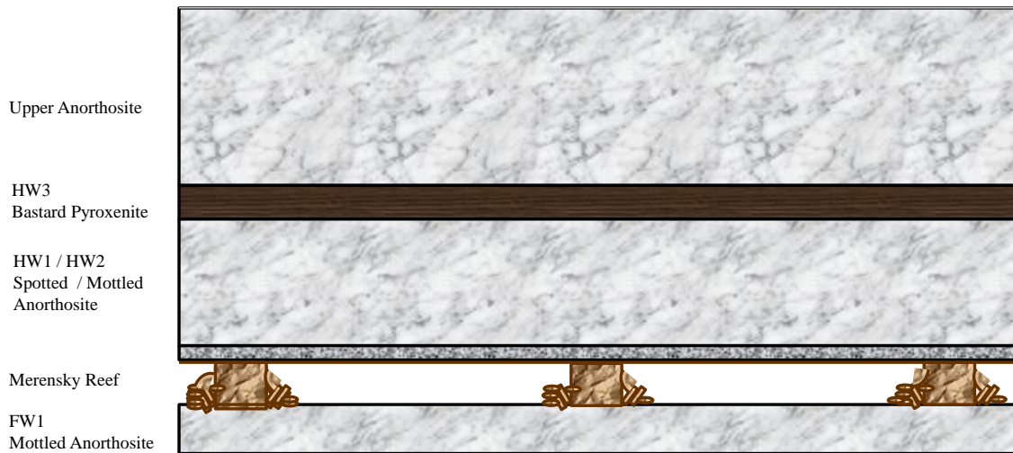
Figure 8.9: Diagram indicating hangingwall stratigraphy. The crush pillars are indicated by the piles of broken rock.
