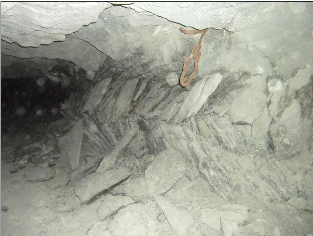
Figure 8.17b: Squeezing Pyroxenitic pillar sidewall.
