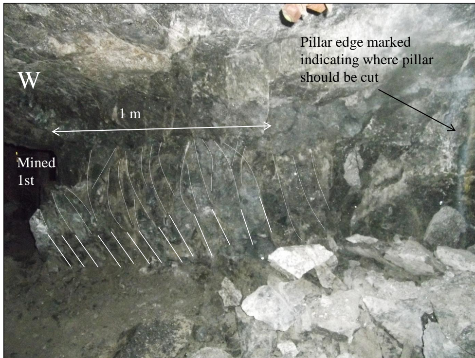
Figure 8.30: Formation of pillar P2 (down-dip view from the holing above the pillar). The face was aligned with the pillar. The fractures are visible along the west side of the pillar (indicated by white traces along the footwall of the pillar). The photograph was taken on 16 March.
