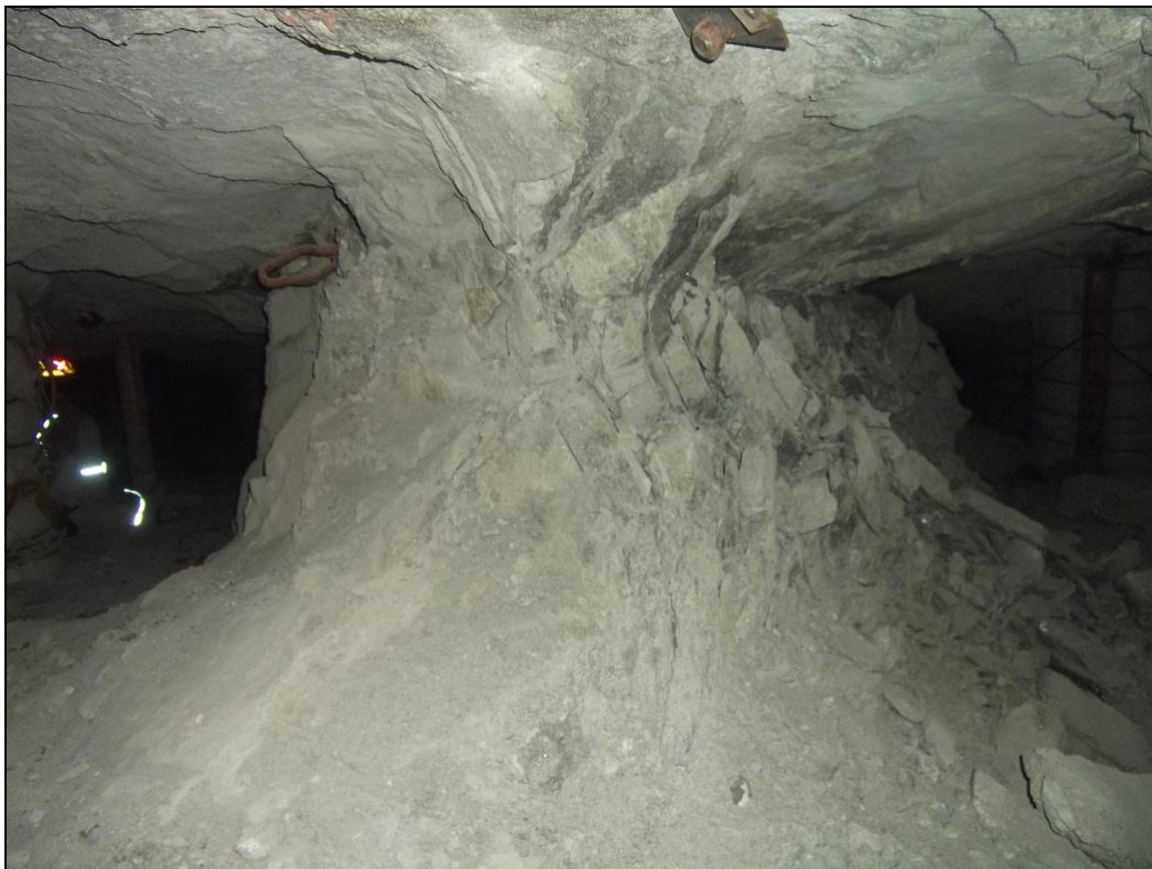
Figure 8.16b: Pillar consisting of Pyroxenite hangingwall (pillar 42).
