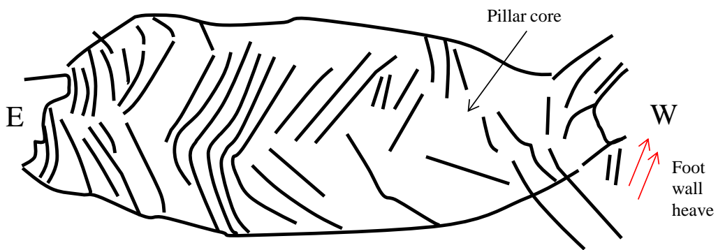
Figure 8.21b: Trace of pillar fractures and orientation.
