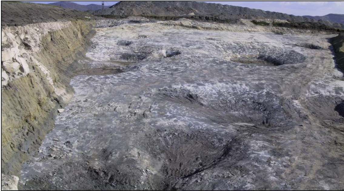
Figure 5.1: Photograph of potholing in a UG2 Opencast operation in the Bushveld Complex.
