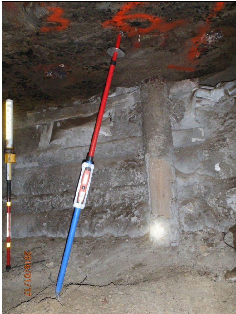
Figure 9.6: Convergence measurement at a closure station using a Dist-o-Rock measuring device.
