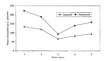
Figure 1 Recovery of Aquasoil® and Stockosorb® polymers after exposure to fertilizer solution. Legend: 1 Distilled water, 2 Tap water, 3 Fertilizer solution, 4 Tap water, 5 Distilled water.
