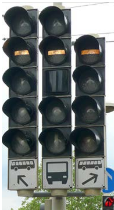
Figures 3a and 3b: Examples of BRT signals with LRT type lenses found in Stuttgart, Germany (Ref 2) and Zurich, Switzerland (Ref 3) respectively
