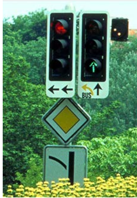
Figures 4a and 4b: Examples of BRT signals similar to normal signals with supplementary signs found in North Kent, England and Schaffhausen, Switzerland (Ref 2)
