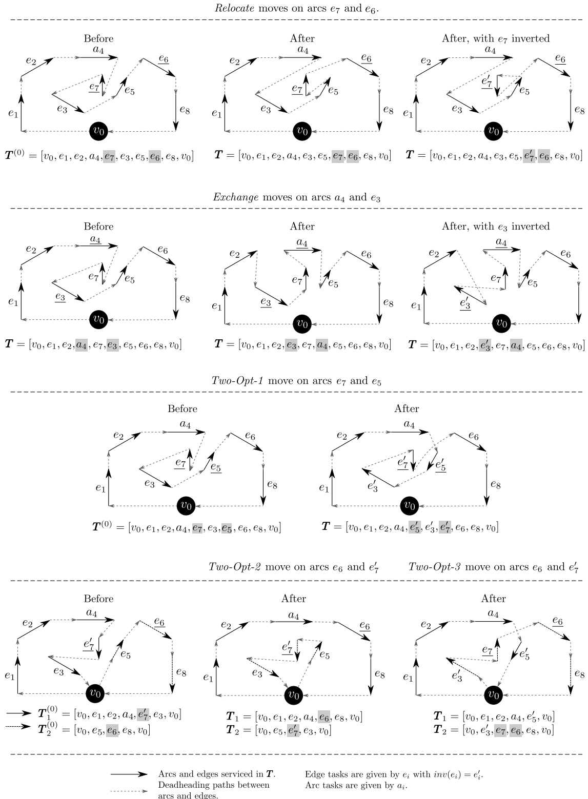
Figure 5.1: Examples of relocate , exchange , two-opt and two-opt-1 move operators for the MCARP.
