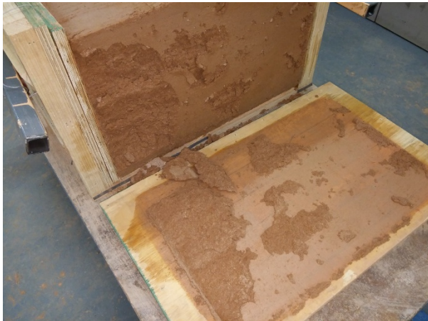
Figure 3.26: Model sides sticking to wooden box panels
