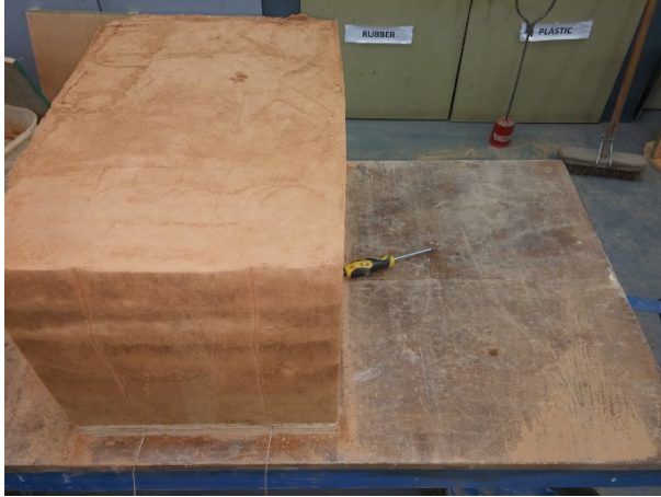
Figure 3.24: Deformation experienced during compaction in the wooden box
