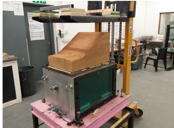
Figure 3.31: Placing embankment in strongbox
