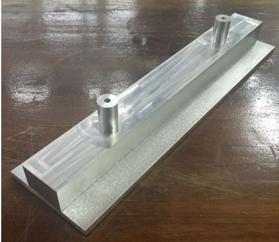
Figure 3.7: Final loading block and plate
