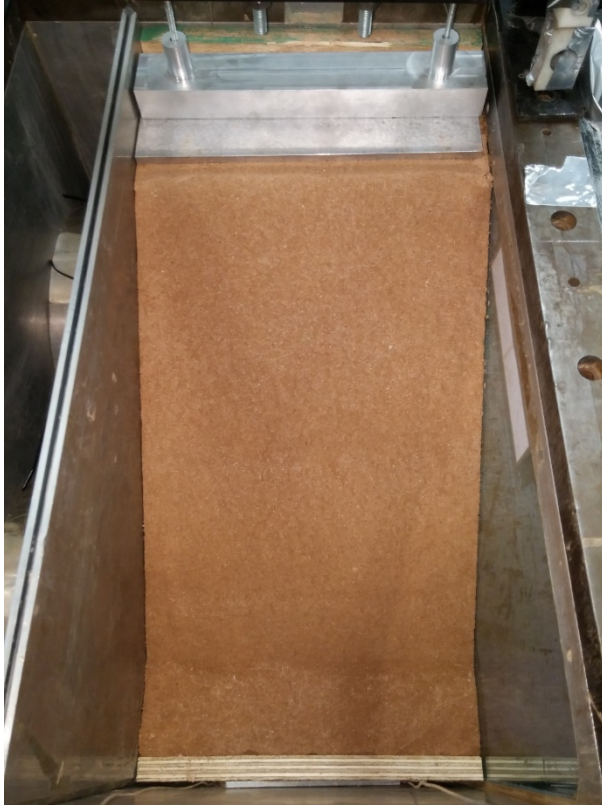
Figure 3.34: Final model setup after compaction outside strongbox
