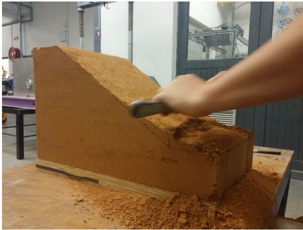
Figure 3.28: Embankment carving process
