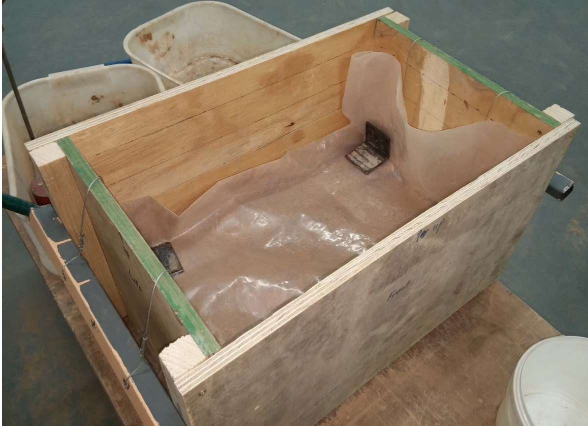
Figure 3.23: Separate wooden box for the compaction process.
