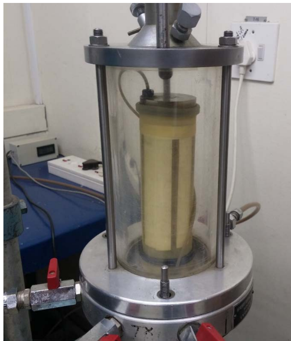
Figure 4.5: Final triaxial setup
