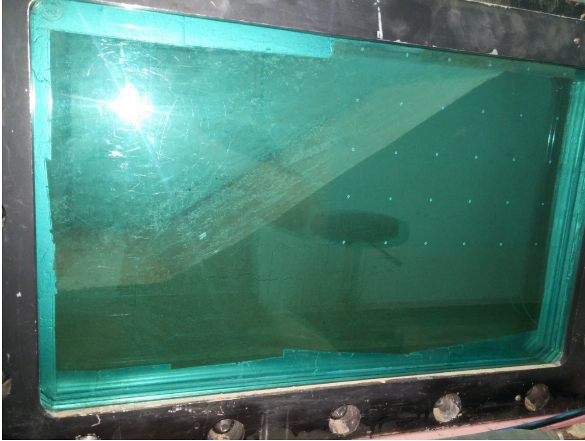
Figure 4.26: Embankment model for Test B6 (23.0 % MC)
