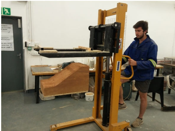
Figure 3.30: Moving embankment with the forklift
