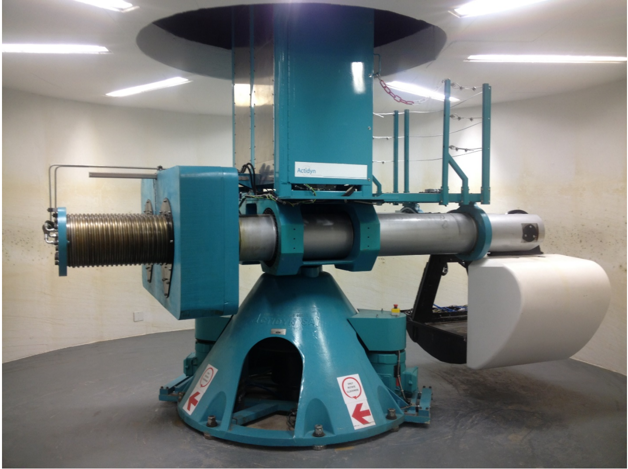
Figure 3.8: Geotechnical centrifuge at the University of Pretoria
