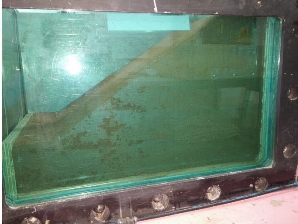
Figure 7.7: Test A2 (20.0% MC - Front of embankment model.
