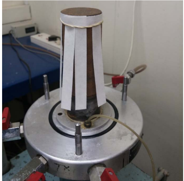
Figure 4.4: Side drains used for the triaxial tests
