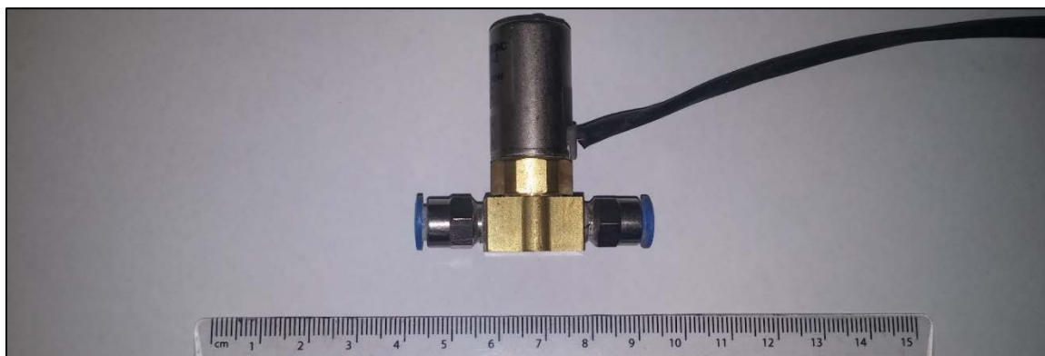
Figure 3.14: Solenoid valve connected to the pneumatic piston
