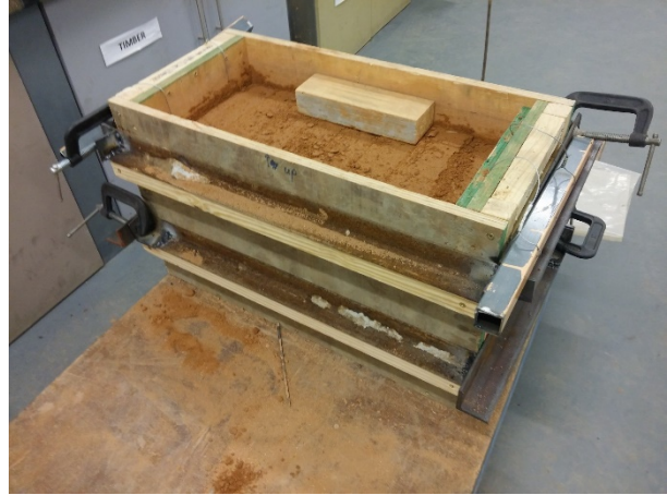
Figure 3.25: Angle profile steel reinforcing to address deformation
