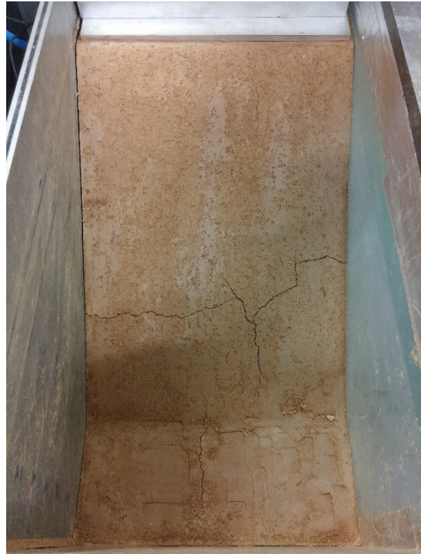
Figure 4.15: Embankment face at the start of Test B3 Figure 4.16: Cracks formed during Test B3.
