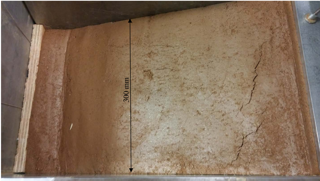
Figure 7.15: Cracks that formed at the top of the embankment for Test A3 (28.0 % MC)
