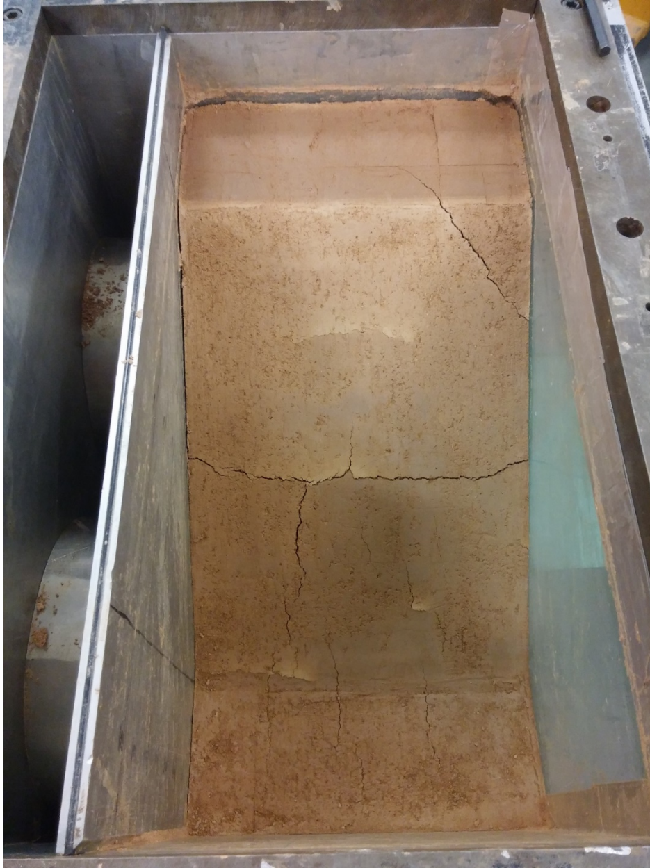
Figure 4.23: Cracks that formed during Test B5 (23.0 % MC)
