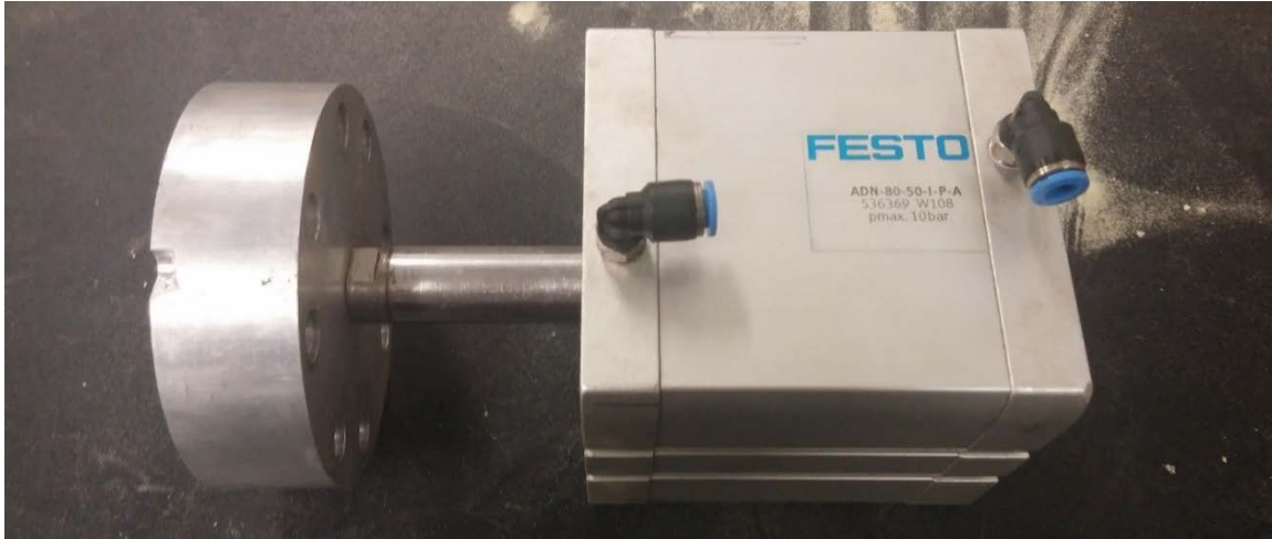
Figure 3.13: Pneumatic piston for load application
