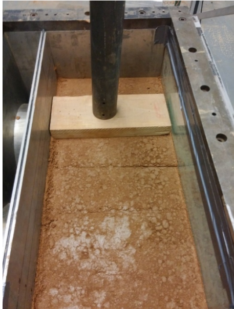
Figure 3.36: Compaction of material
