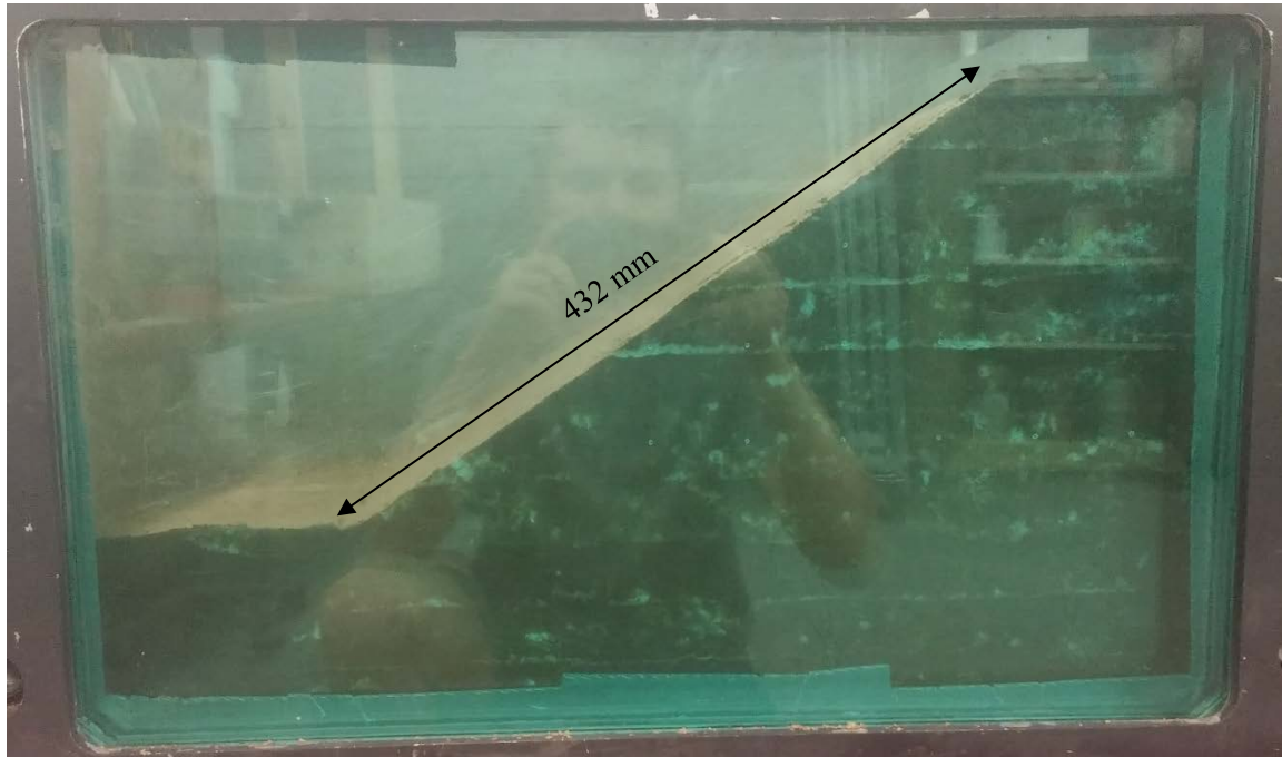
Figure 4.10: Front of embankment for Test B1 (21.0 % MC)
