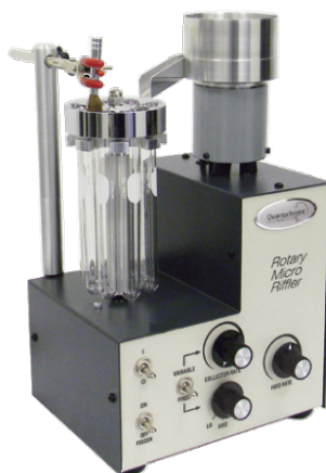
Figure 7.1: Rotary micro riffler. (Quantachrome 2014)
