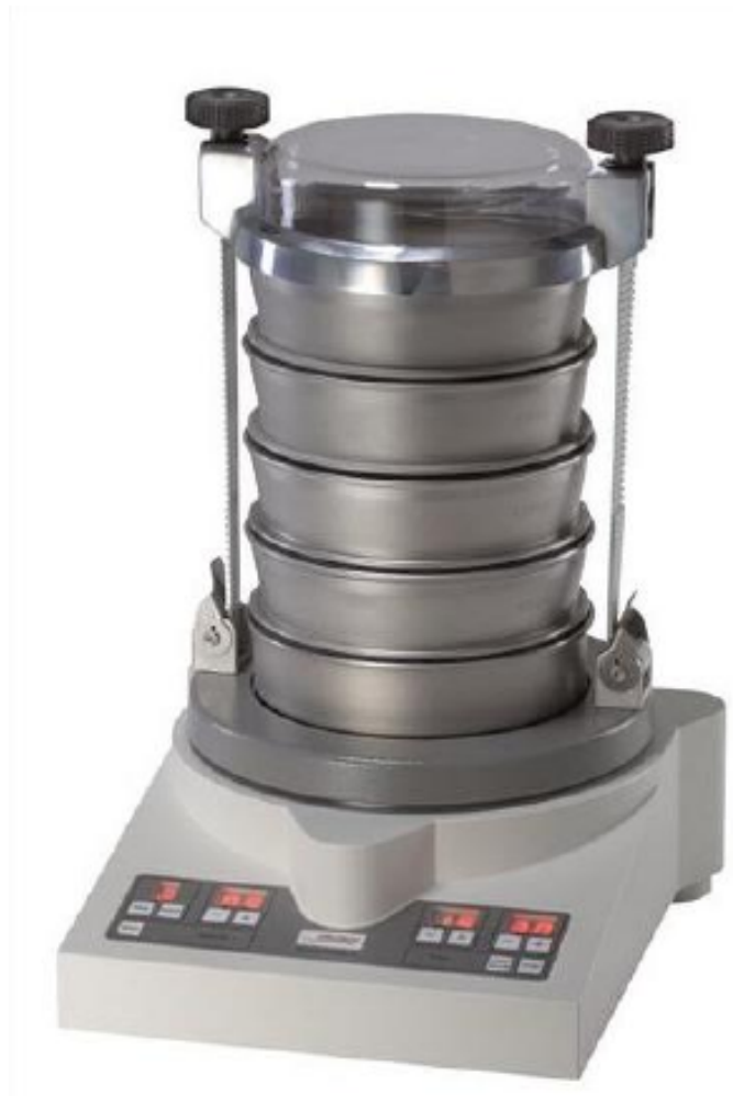
Figure 2.41: A laboratory sieve shaker to determine particle size distribution. (Fritsh 2014)
