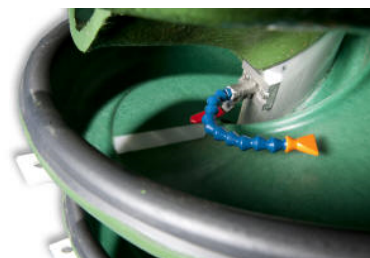
Figure 2.10: Wash water addition point. (Multotec 2014b)
