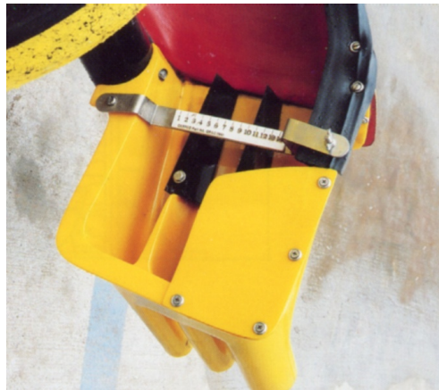
Figure 2.16: Example of a product splitter box - concentrate on inside for high-density valuable product. (Mine Engineer 2014)
