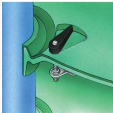
Figure 2.8: Auxiliary side splitter. (Multotec 2014a)
