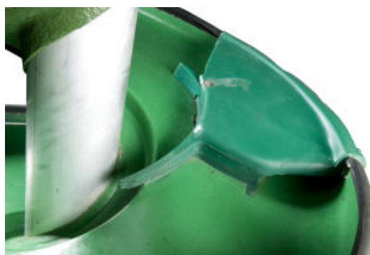
Figure 2.6: Repulper design on a single spiral start. (Multotec 2014b)
