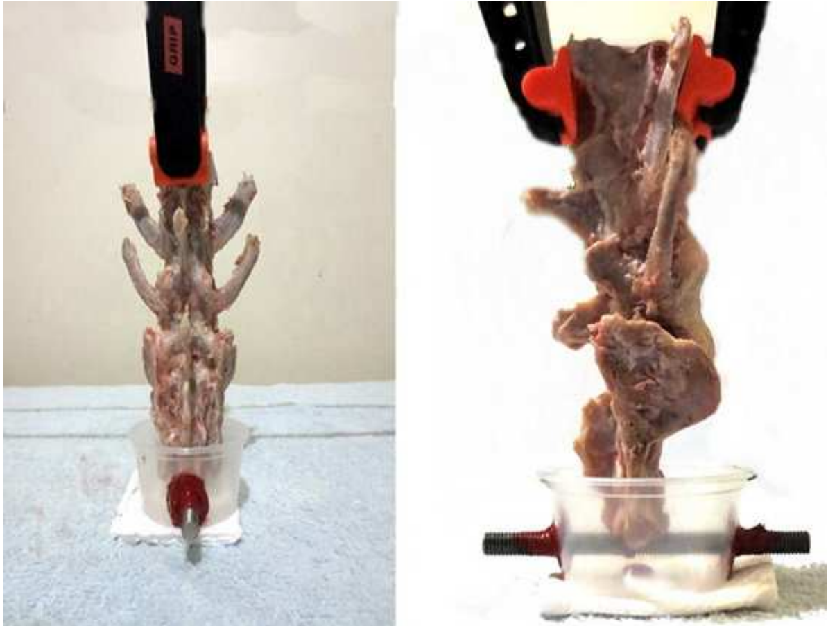
Figure 3.19: Dorsal and lateral views of potting and alignment by visual means of the sacral end of each bony specimen.
