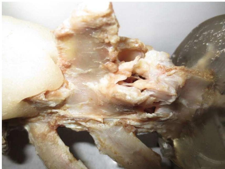
Figure 4.4: Photo of failure of the L5-L6 joint (pin-PMMA).
