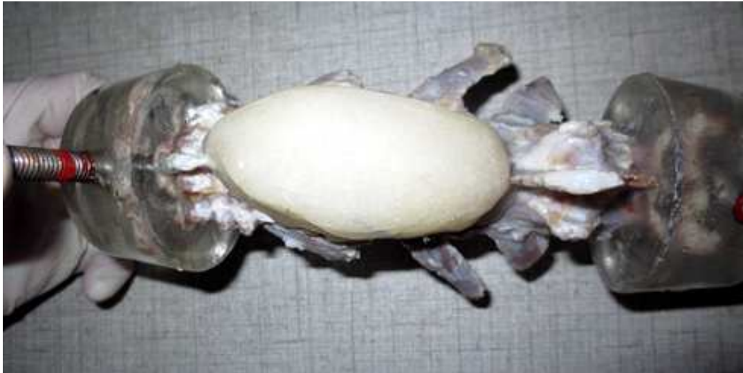
Figure 3.8: Photo of the dorsal view of the pin-PMMA placement. The cranial end (L5) is to the right and the sacrum is to the left in this image.
