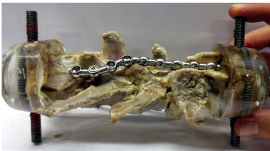
Figure 3.14: Photo of the lateral view of the SOP placement. The cranial end (L5) is to the left and the sacrum is to the right in this image. Note how the SOP plates are bent along the contours of the vertebrae to obtain an optimal fit.
