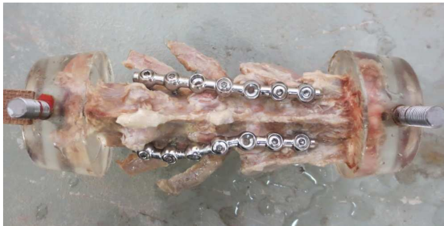
Figure 3.13: Photo of the dorsal view of the SOP placement. Stabilisation was performed using 3.5 mm SOP Locking plates (Orthomed UK Ltd, Halifax, UK) bilaterally, with 3.5 mm cortical screws were anchored in the L6, L7, S1 and S2 vertebral bodies. The cranial end (L5) is to the left and the sacrum is to the right in this image.
