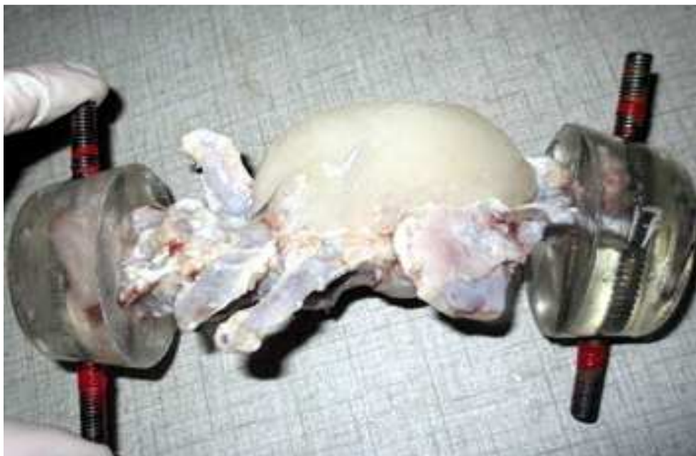
Figure 3.9: Photo of the lateral view of the pin-PMMA placement. The cranial end (L5) is to the left and the sacrum is to the right in this image.
