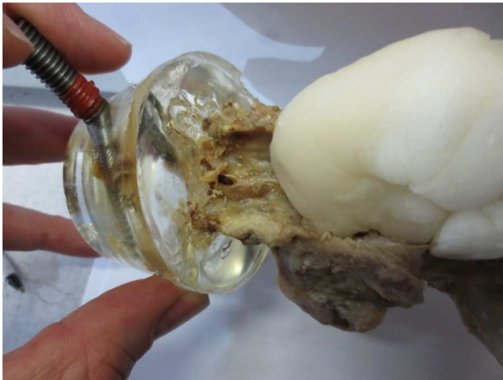
Figure 4.12: Photo of failure of the connection between the epoxy and the sacrum (MoF4).
