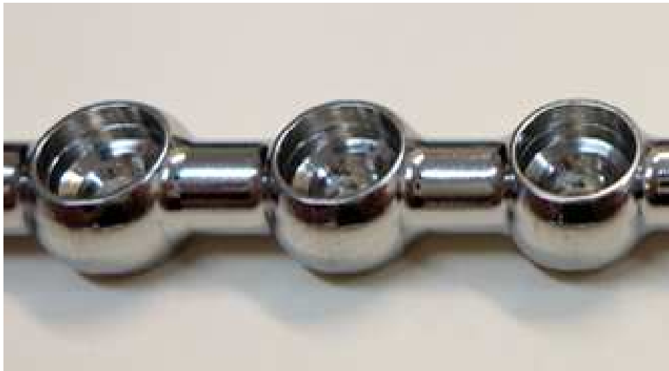
Figure 2.3: Close-up view of a SOP Interlocking Plate. The top of the node is wider, allowing a standard cortical screw to recede into the plate when tightened. The base of the node portion contains a threaded portion, causing a press fit of the screw in the node.
