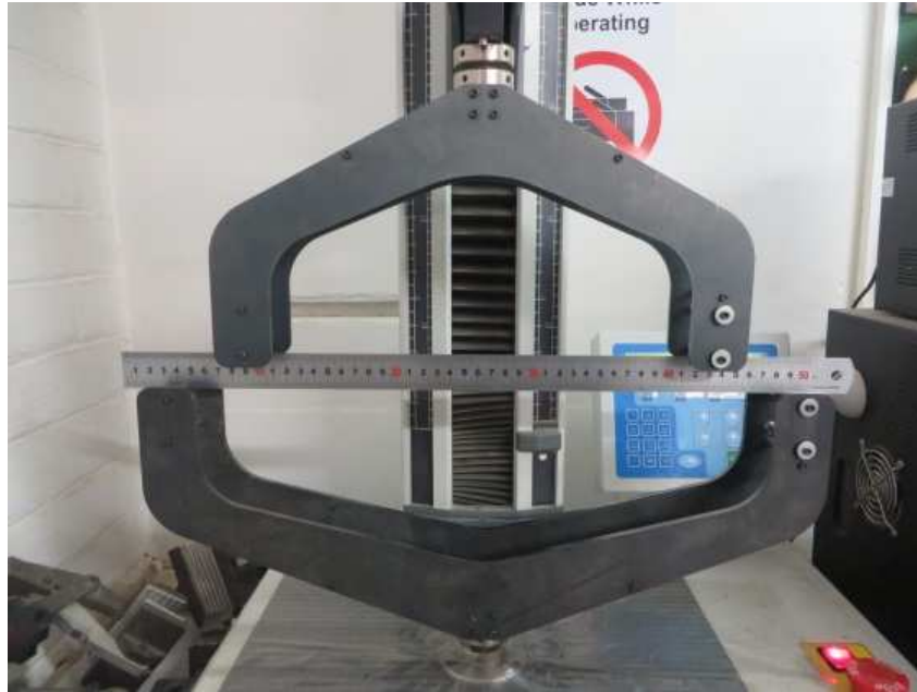
Figure 3.21: Alignment of top and bottom jaws of the FBC-SLS. A steel ruler was used to align the top and bottom jaws of the FBC-SLS.
