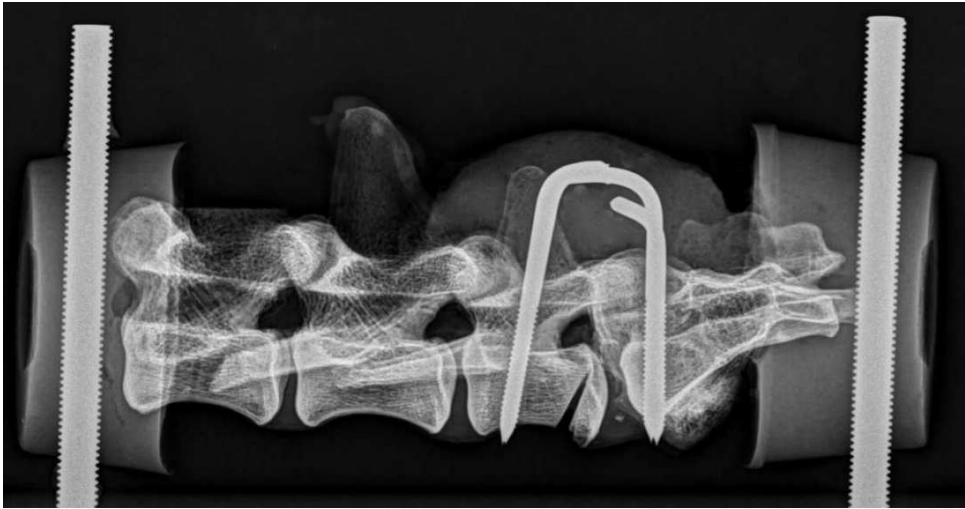
Figure 3.10: Lateral radiographic view of the pin-PMMA placement. The cranial end (L5) is to the left and the sacrum is to the right in this image.
