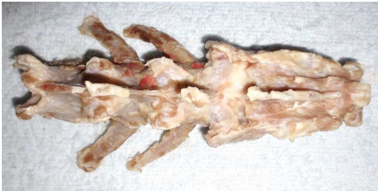
Figure 3.1: Dorsal view of typical test specimen (L5–S3), before potting cranial and caudal ends in epoxy. The spinous process and both transverse processes of L5 were removed to facilitate potting of the specimens in the epoxy. The cranial end (L5) is to the left in this image.
