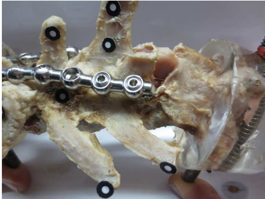
Figure 4.5: Photo of failure of joint L5-L6 in a SOP specimen.
