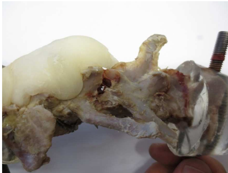
Figure 4.7: Photo of failure of joint L6-L7 joint in a pin-PMMA fixated bony specimen.
