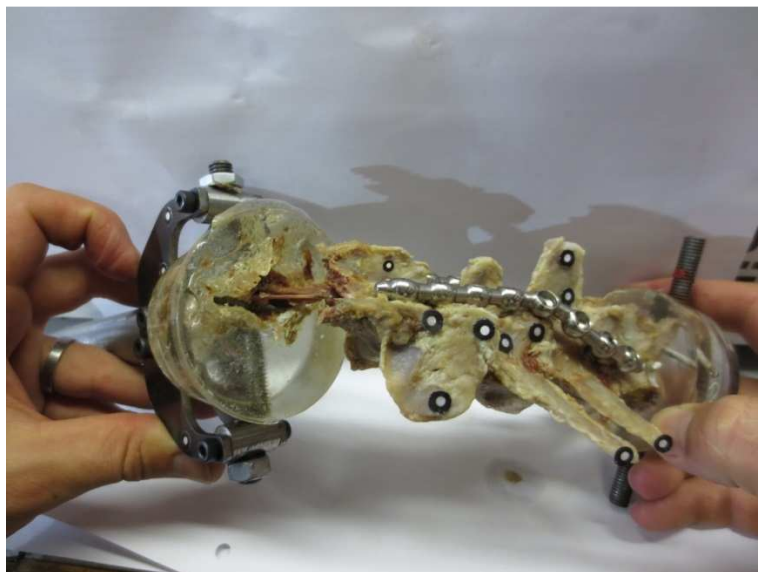
Figure 4.10: Photo of failure (fracture) of a sacrum at the sacrum-epoxy interface (SOP specimen).
