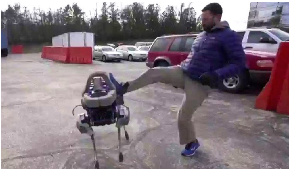
Figure 14: Screen shot from Introducing Spot , where an employee kicks a robotic dog in order to prove its stability (Boston Dynamics 2015).
