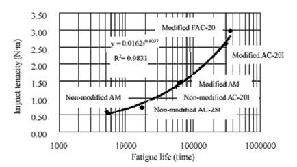
Figure 4. The relationship of fatigue life and impact tenacity.
