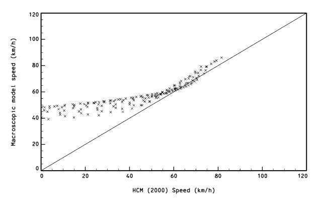
Comparison of HCM (2000) and Macroscopic model speeds Specific upgrade segments: 6.5% Gradient, 3.7m Lane, 0.5m Shoulders
