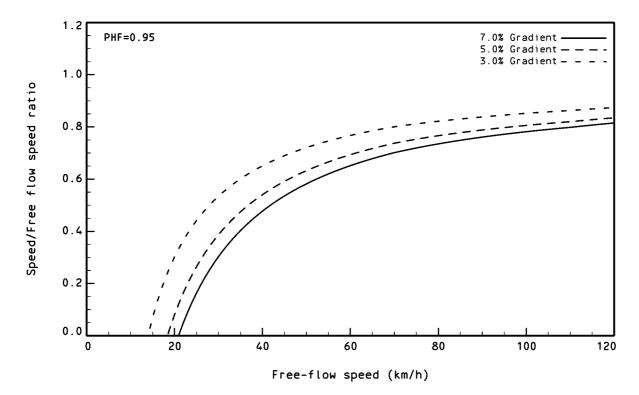
Impact of free-flow speed 1.00 km Grade length For 800 Veh/h Flow, 10% Heavies, 60/40% Split, 20% No-passing
