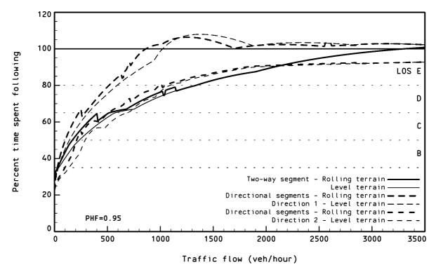
Impact of traffic flow - 100 km/h Free-flow speed For 10% Heavies, 80/20% Split, 80% No-passing
