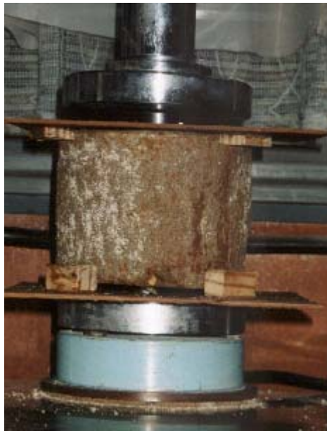
Plate 1. Position of specimen in double punch tensile test.
