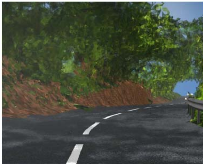
Figure 10. Rendered image of embankment with vegetation extracted directly from laser scan data.
