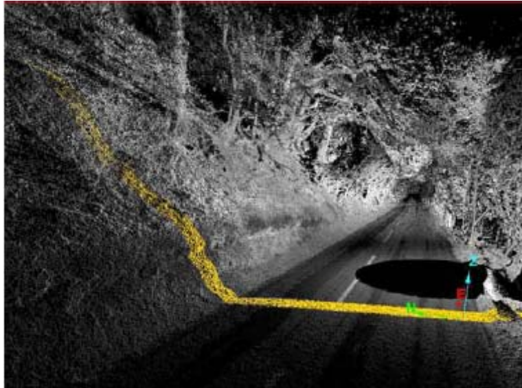
Figure 6. Laser scan data of an incident site involving a vehicle rollover, example cross-section highlighted.
