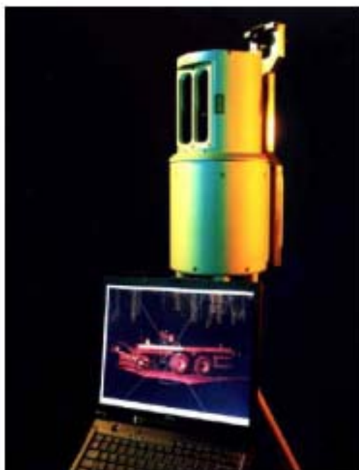
Figure 1. RIEGL LMS-Z210 laser scanner, and the ISiTE 3D analysis software.
