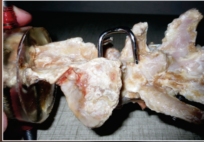
Figure 2: The pins were bent to achieve maximum overlap of caudal, lateral, right, and left pins at a level just below the dorsal spinous processes' dorsal edge. PMMA was applied dorsally to bond all the pins, articular facets and dorsal spinous processes of L7 and S1.
