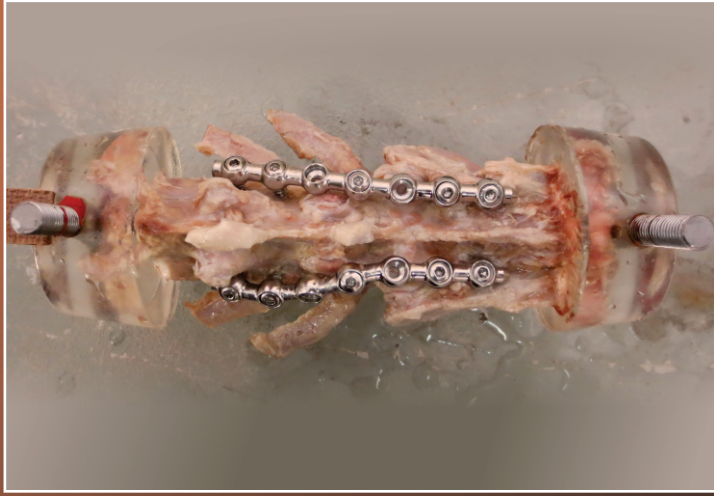
Figure 1: Stabilization was performed using 3.5 mm SOP Locking plates (Orthomed UK Ltd, Halifax, UK) bilaterally, with 3.5 mm cortical screws anchored in the L6, L7, S1 and S2 vertebral bodies.
