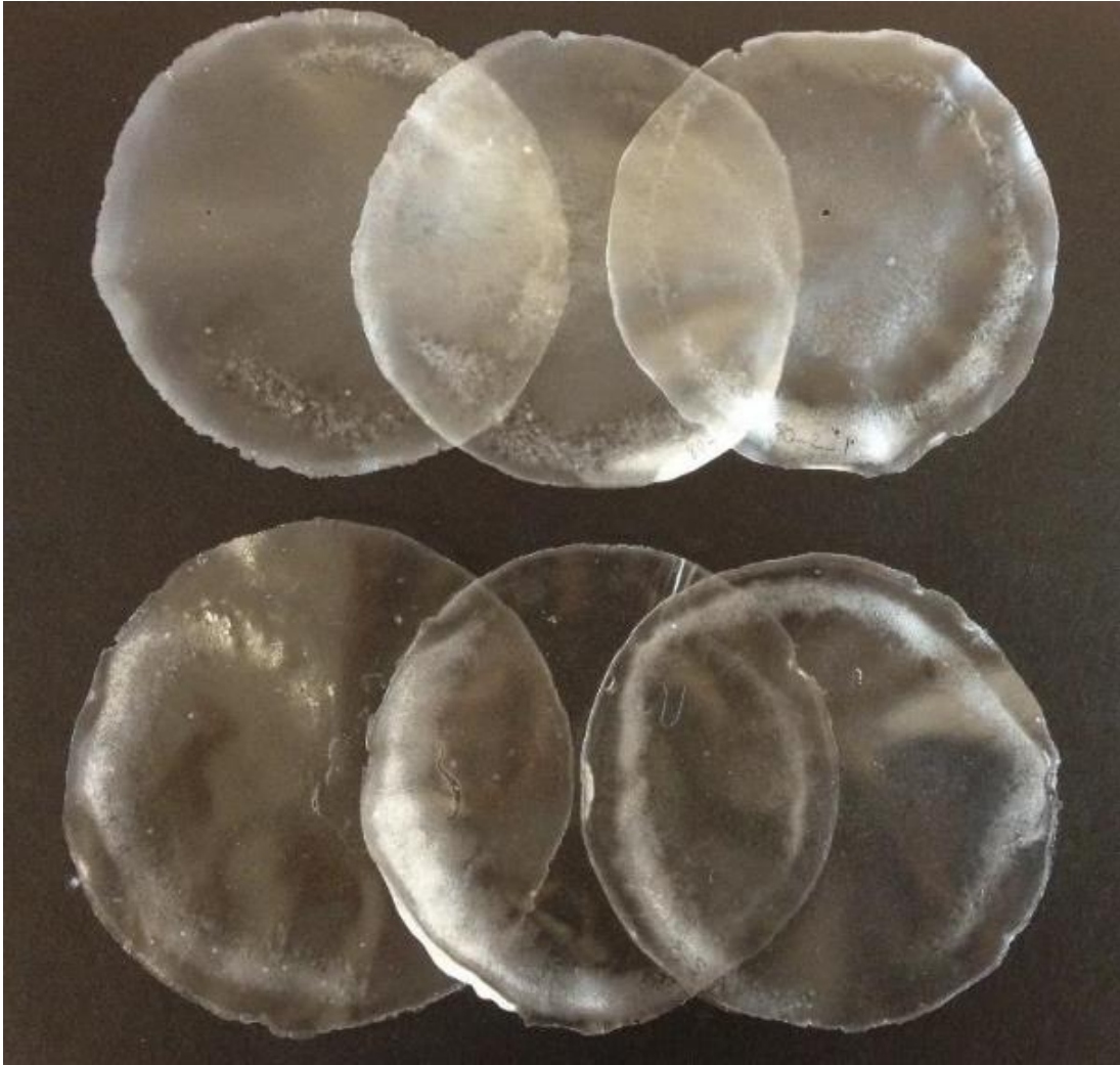
Figure 6-1: Improved transparency of the films when regeneration and rinsing is performed at 25 °C (bottom) compared to regeneration and rinsing at 80 °C (top).
