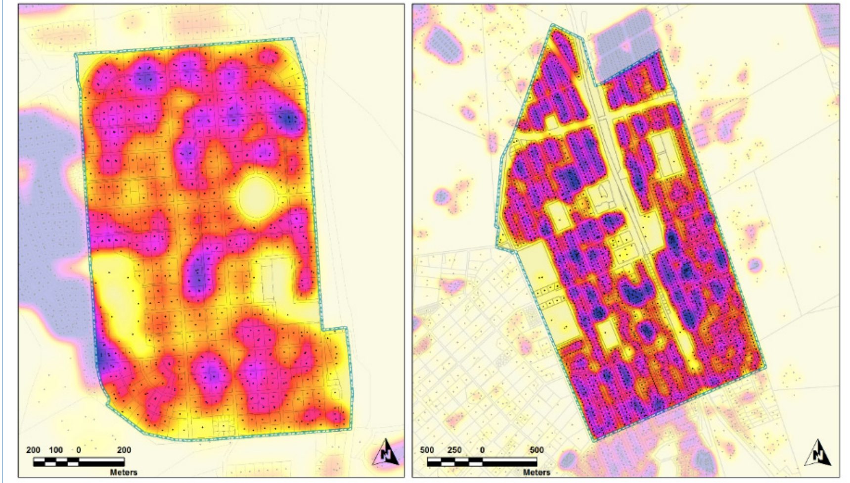
Kernel Densities: 100m (Densities derived from ESKOM SPOT Building Count 2012 using ArcGIS kernel density function)
