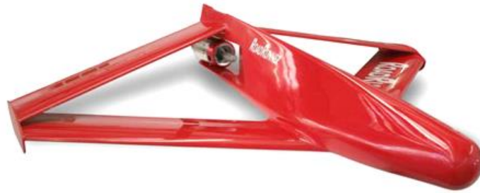
Figure 1.1: PAT Roadrunner UAV with turbine engine
