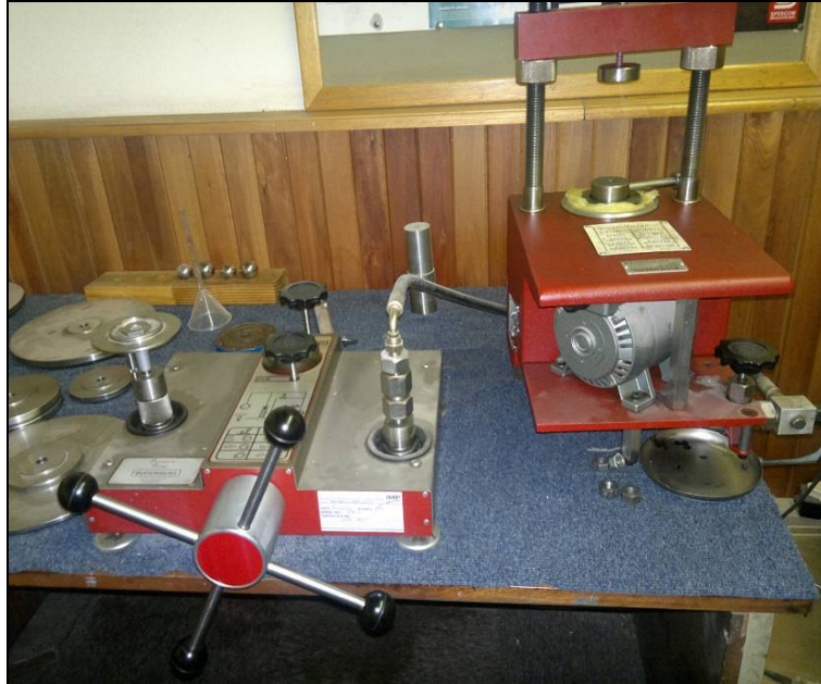
Figure 3.5: Dead weight standard Budenberg calibration system
