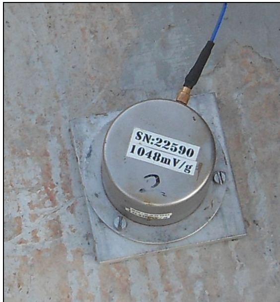
Figure 3.6: Accelerometer 1 fixed on surface of footing using an aluminium block.
