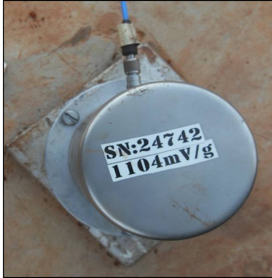
Figure 3.7: Accelerometer 2 fixed on surface of footing using an aluminium block
