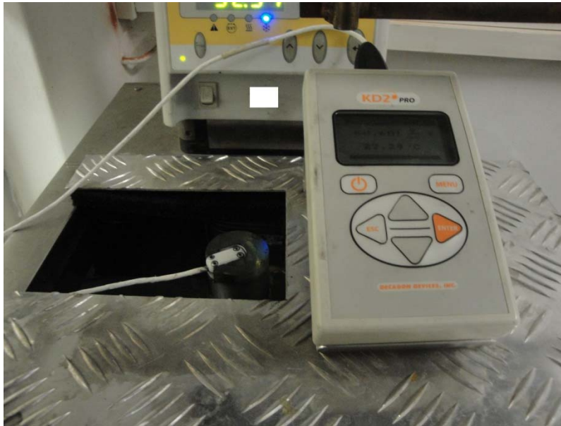
Figure 3-5: KD2 Pro with probe in nanofluid sample in water bath
