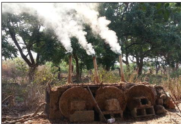
Figure 5. Wood drying stage of carbonisation
