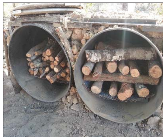
Figure 3. Logs loaded longitudinally LHS and crosswise RHS in drum Kilns
