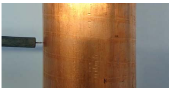
Figure 3 Image showing the constantan needle measuring the tube wall temperature.
