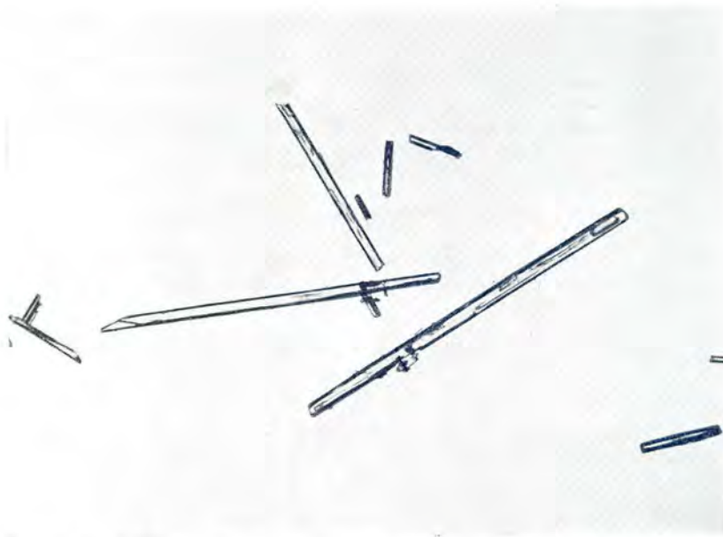
Fig. 2.—Methyl ester of monocarboxylic dilactonic acid m.p. 190-191°; \times 50 .
