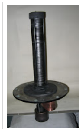
Figure 2.6: Main cavity of the black body, consisting of graphite rings
