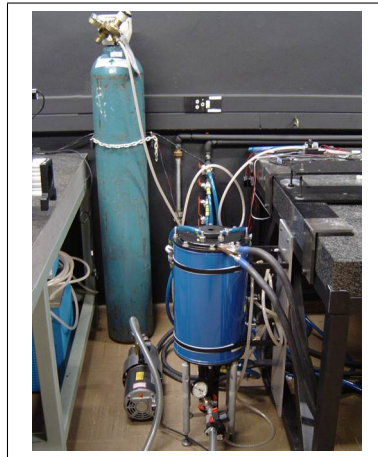
Figure 2.7: Black body operated in a vertical position while filling the crucible with the eutectic alloy
