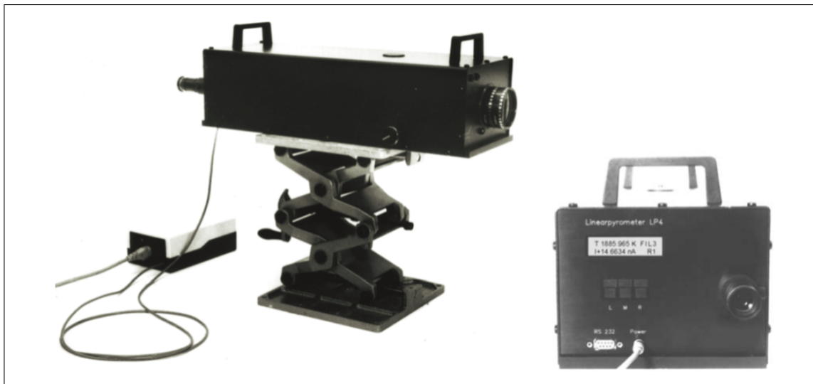
Figure 2.9: A picture of the NMISA's LP4 radiation thermometer supplied by IKE (Stuttgart, Germany)
