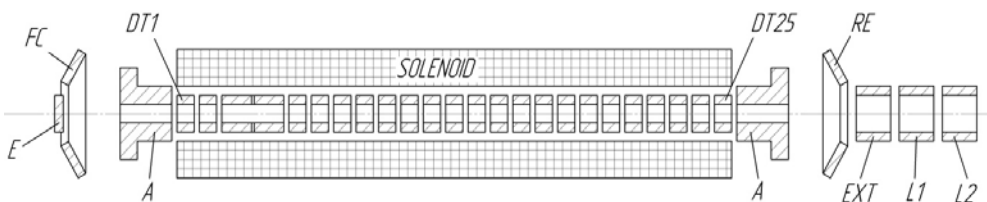
Figure 3.1: A schematic diagram of the Krion-2 ESIS: (a) electron emitter (E), (b) false-cathode electrode (FC), (c) surrounding emitter, (d) anodes (A) (electron gun anode –left, electron reflector anode – right), (e) sectioned cylindrical drift tubes (DT1-DT25) are arranged inside the bore of a superconducting solenoid with B_{max} = 3 Tesla, (f) electron reflector (RE) with an orifice at the centre for the ions extraction; (g) focusing electrostatics lenses (EXT,L1 and L2) for ion beam extraction and focusing. The total length of the ionization trap between DT1 and DT25 is 120 cm. The axial symmetry and geometrical axis of the system coincides with the magnetic axis of the solenoid with a precision better than 0.1 mm.
