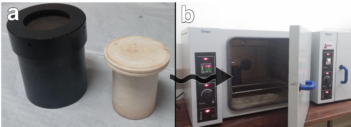
Figure 3-3 Complete system for the hydrothermal chemical growth; (a) shows the stainless steel autoclave system with the Teflon lining (b) shows the electric oven used for heating
