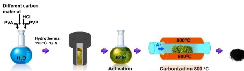
Scheme 1. Schematic diagram of the preparation process of activated carbons.
