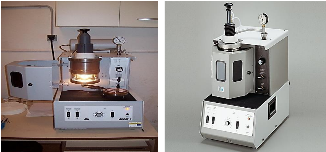
Figure 3.1: The Compact Arc-Melter (Edmund Bühler GmbH MAM-1) at the University of Pretoria.
