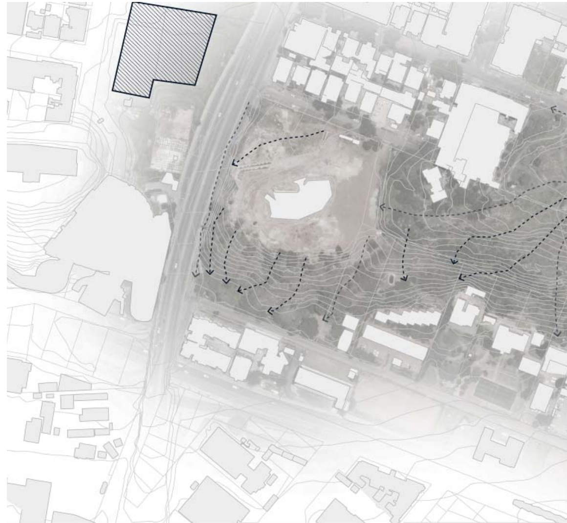
fig 4.36. Mapping of potential water runoff directions and flows as the site is the watershed between north- and east-flowing rivers that end up in the Indian Ocean, and south- and west-flowing rivers which end up in the Atlantic Ocean
