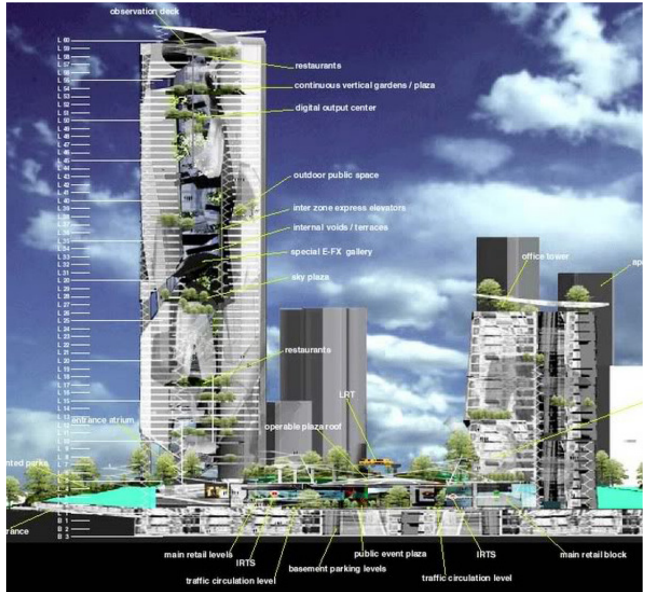
3.12_ Diagram of the EDITT Tower ( https://archiandesigns.files.wordpress.com/2014/08/editt-tower-singapore-by-the-architect-ken-yeang-of-malaysia-3.jpg )
