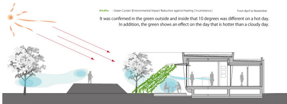
8.24_ Diagram illustrating the passive design ( http://www.archdaily.com/421607/green-screen-house-hideo-kumaki-architect-office/521e4e27e8e44ed7fc00003a-green-screen-house-hideo-kumaki-architect-office-diagram edited by author, 2015)
