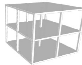
Infrastructure as skeleton This form of infrastructure (support) includes load bearing elements and access which includes galleries and cores.
