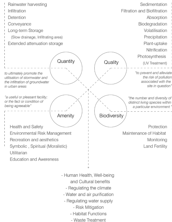
Figure 4.6: The four primary components of integrating urban stormwater strategies
