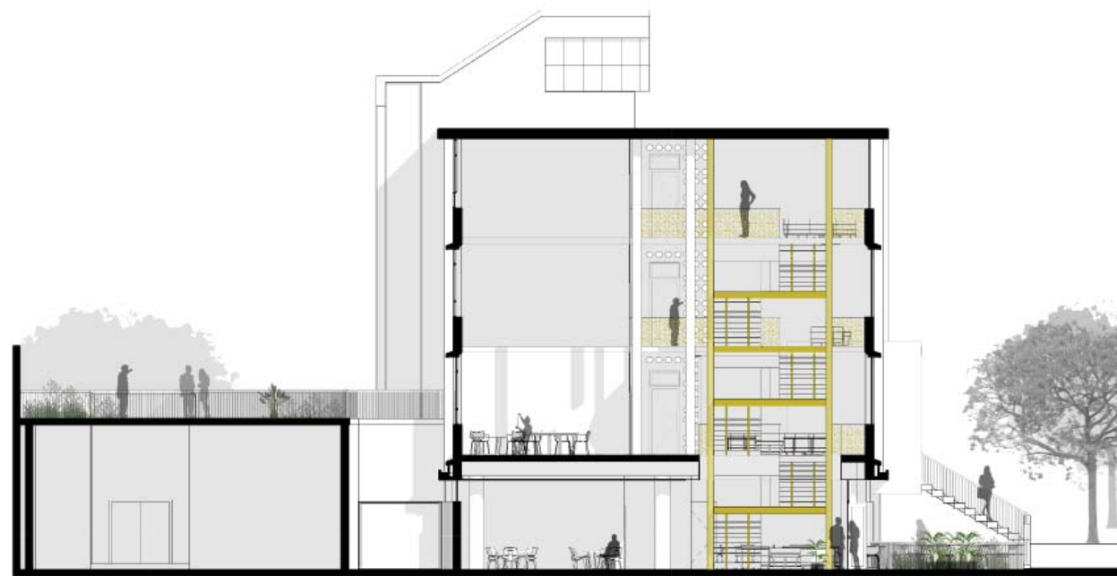
Figure 4.32 Conceptual section as presented in June showing the proposed staircase intervention and new entrance.
