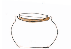
6. Dry plaster container to drain extra water
