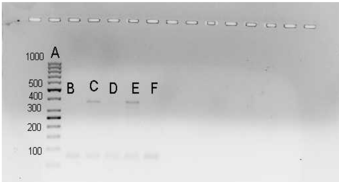
Figure 3.1: Allele specific PCR gel with Roche master mix showing faint bands and non-specific amplification bands between 50 and 100 bp
