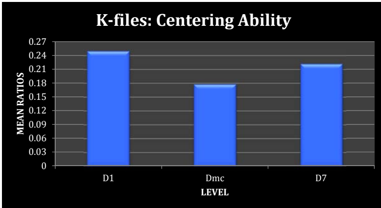
Figure 4.1: Mean centering ratios of the stainless steel K-files at D1 (1 mm from the apical foramen), D mc (point of maximum curvature) and D7 (7 mm from the apical foramen)
