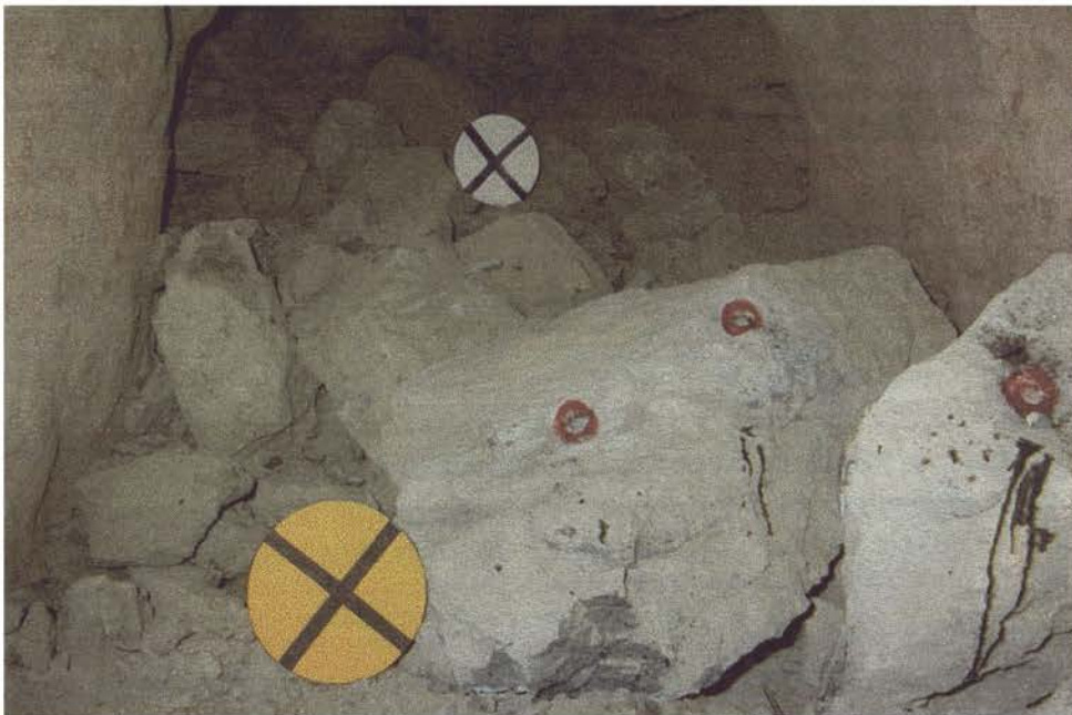
P.8.5. High Hangup with single large fragment across throat of drawpoint
