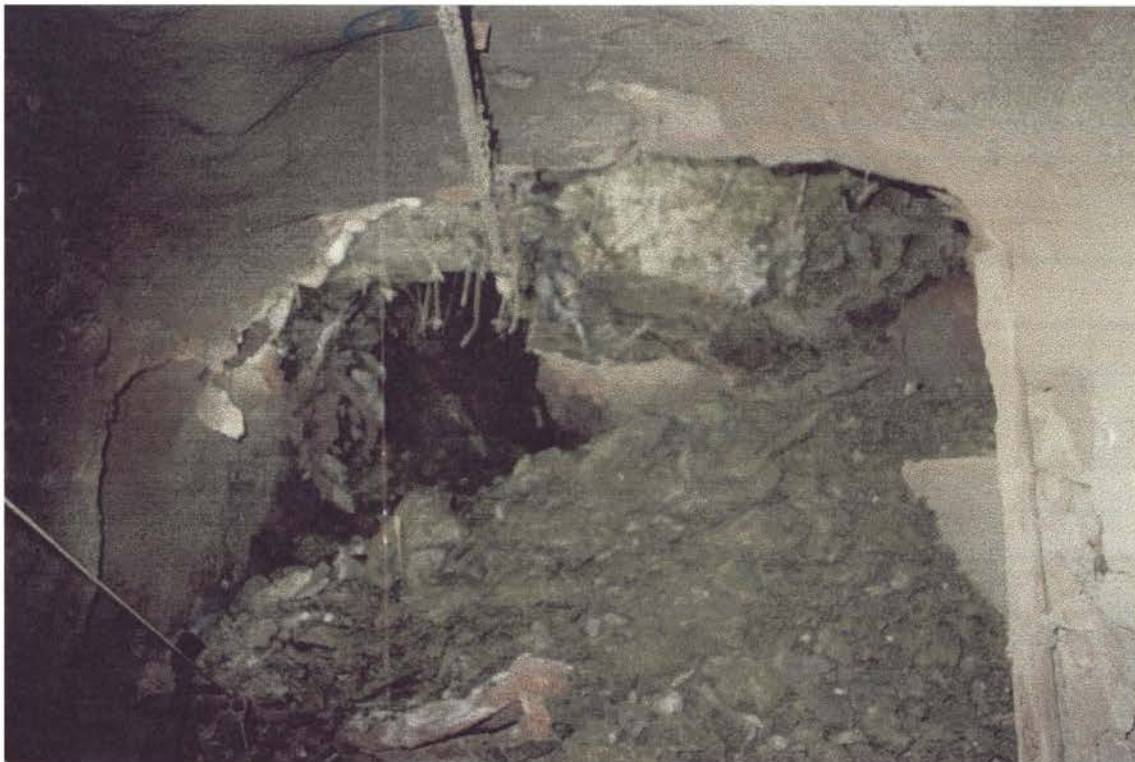
P.A. 15. Tuffisitic Kimberlite Breccia after it has been affected by water (MRMR 20).
