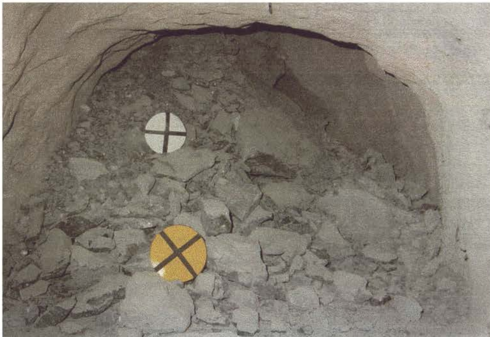
P.8.3. Fragmentation in Hypabyssal Kimberlite drawpoint after 30 000 tons drawn
