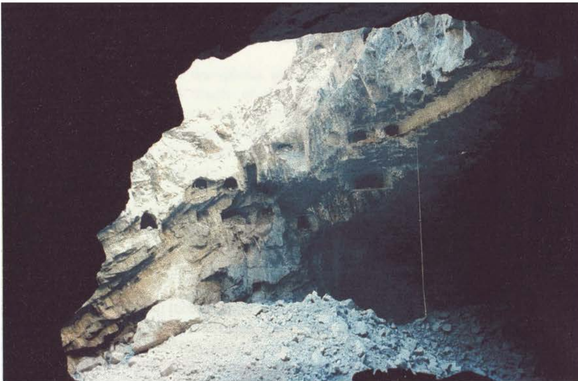
P.8.2. Primary fragmentation into top of ore column after collapse of sill
