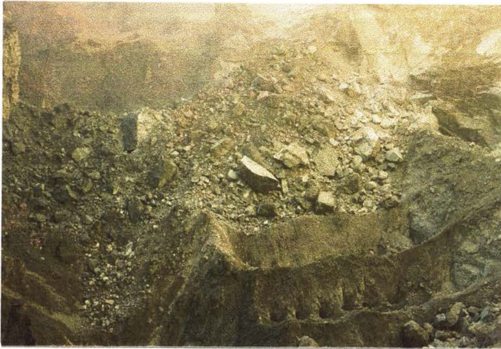
P.9.1. Continuous troughs and drawpoints exposed in glory hole
