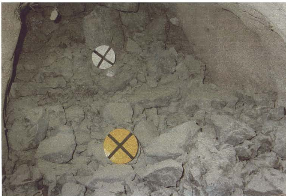
P.8.4. Fragmentation in drawpoint in Tuffisitic Kimberlite Breccia after 30 000 tons drawn
