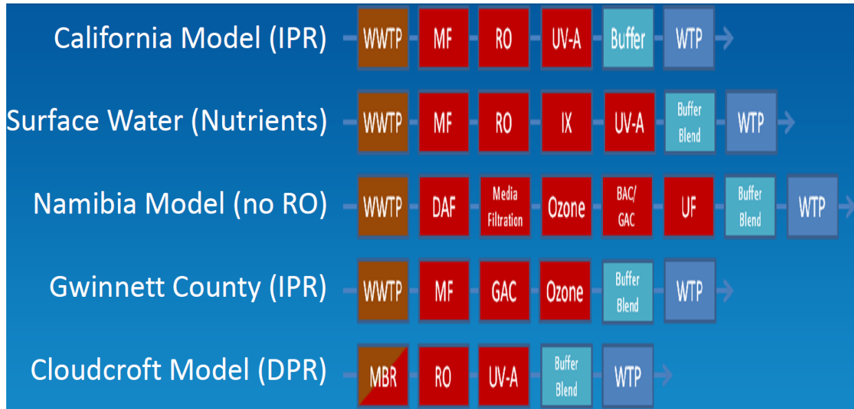
Figure 5.20: Typical treatment process trains (Chalmers et al. , 2011)
