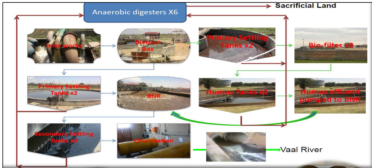
Figure 3.12: Process flow diagram of WWTP3 (Rand Water, 2013)
