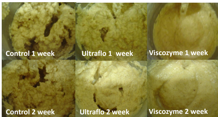
Figure 4.1.3: Effects of treatment with Viscozyme and Ultraflo on cassava slurry viscosity after 1 week and 2 weeks incubation
