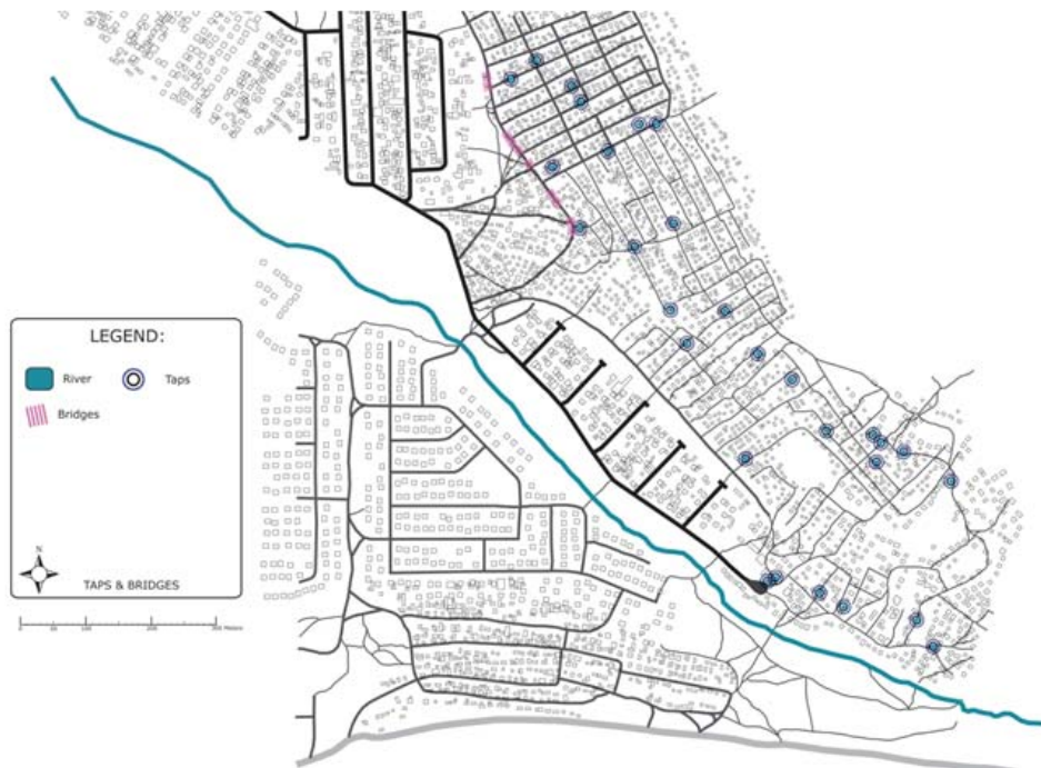
Figure 5.41 : Documentation of existing illegal water connections in the Alaska informal settlement (Rossi 2011)
