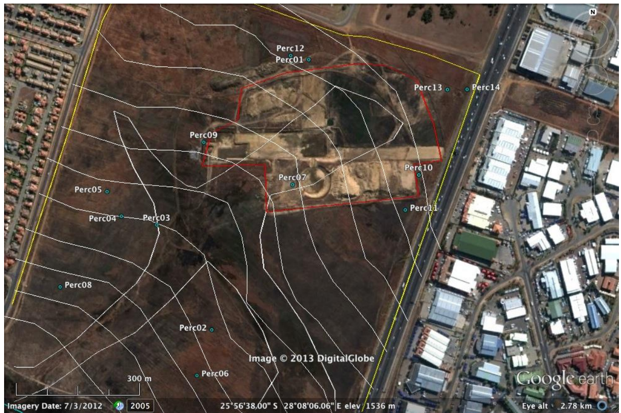
Figure 14. Positions of fourteen percolation tests depicted on surface contours inferred from Google Earth (© 2013); north-eastern contour 1 550 mamsl, decreasing by 5 m intervals to 1 500 mamsl in the southwest.
