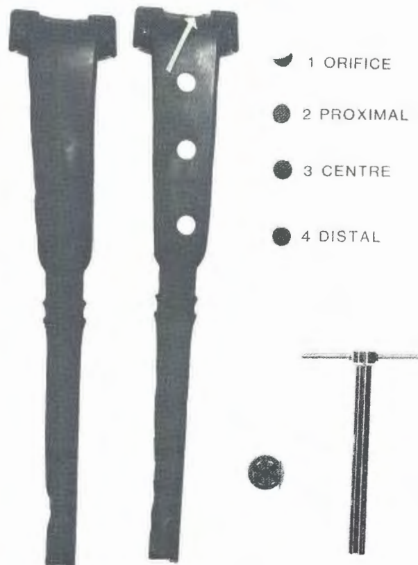
FIG. 1 Halves of teat cup liner (left not sampled; right sampled); sample No. 1 and 2-4 excised from orifice and respectively proximal, central and distal third of liner wall; cork borer; small sample bottle viewed through its bottom towards star-shaped portion of stopper
