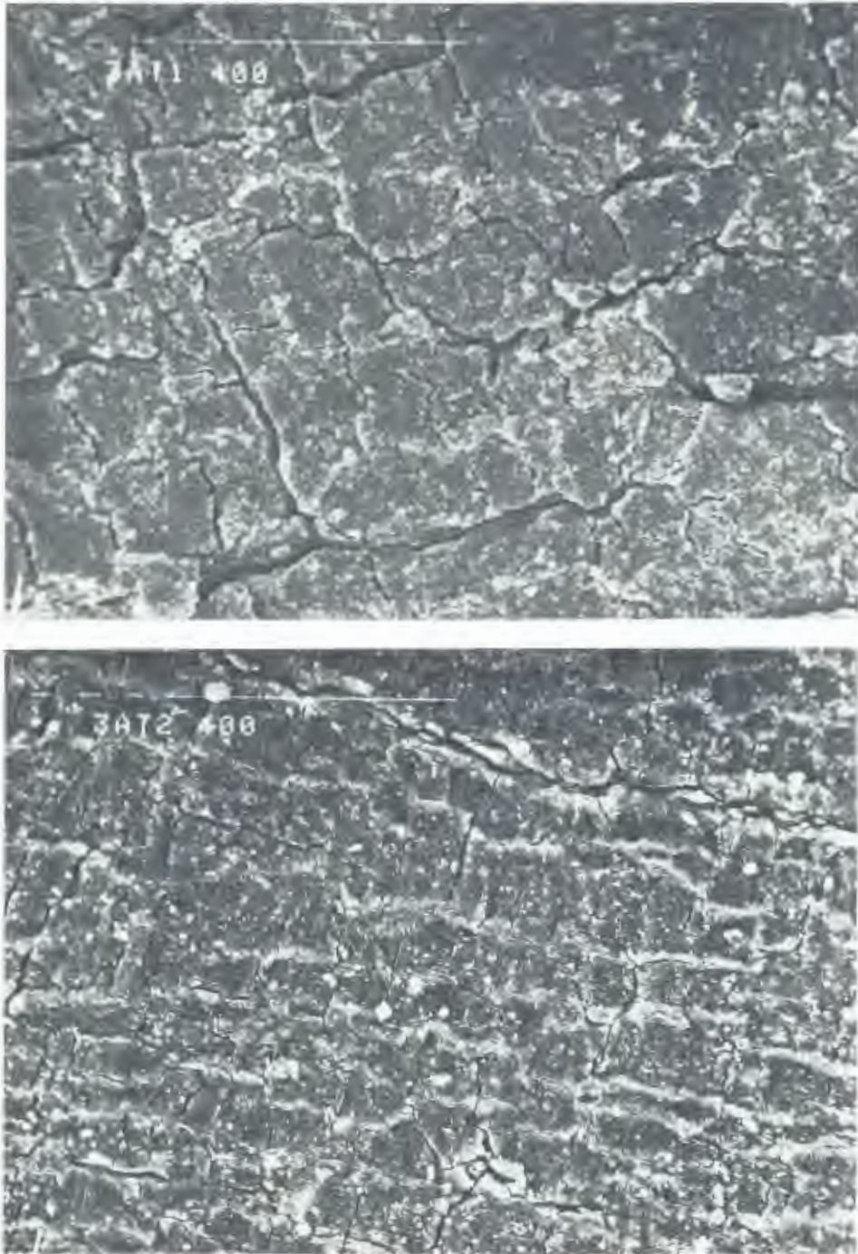
FIG. 18 The surface after 500 milkings of the same liner (i.e. used liner 3A) investigated at the orifice (top) and proximal third (bottom) of liner wall
