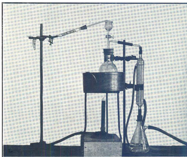
Fig. 3.—Apparatus for determination of volatile acid in alkaline hydrolysis of cucumin.
