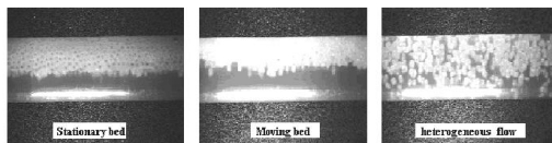
Figure 2 Flow pattern of the paraffin slurry for 6% particles mass fraction
