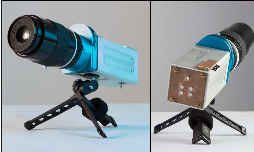
(a) The working solar-blind UV-sensitive electro-optic demonstration device (left) with LED indicators at the back (right).
