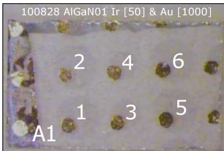
(b) The barely visible \text{IrO}_2 Schottky contacts were formed after annealing the \text{Ir} Schottky contacts at 700°C under \text{O}_2 ambient for 20 minutes. Thereafter, six circular 0.30 mm-diameter, 1000 Å-thick \text{Au} probe contact pads were deposited.
