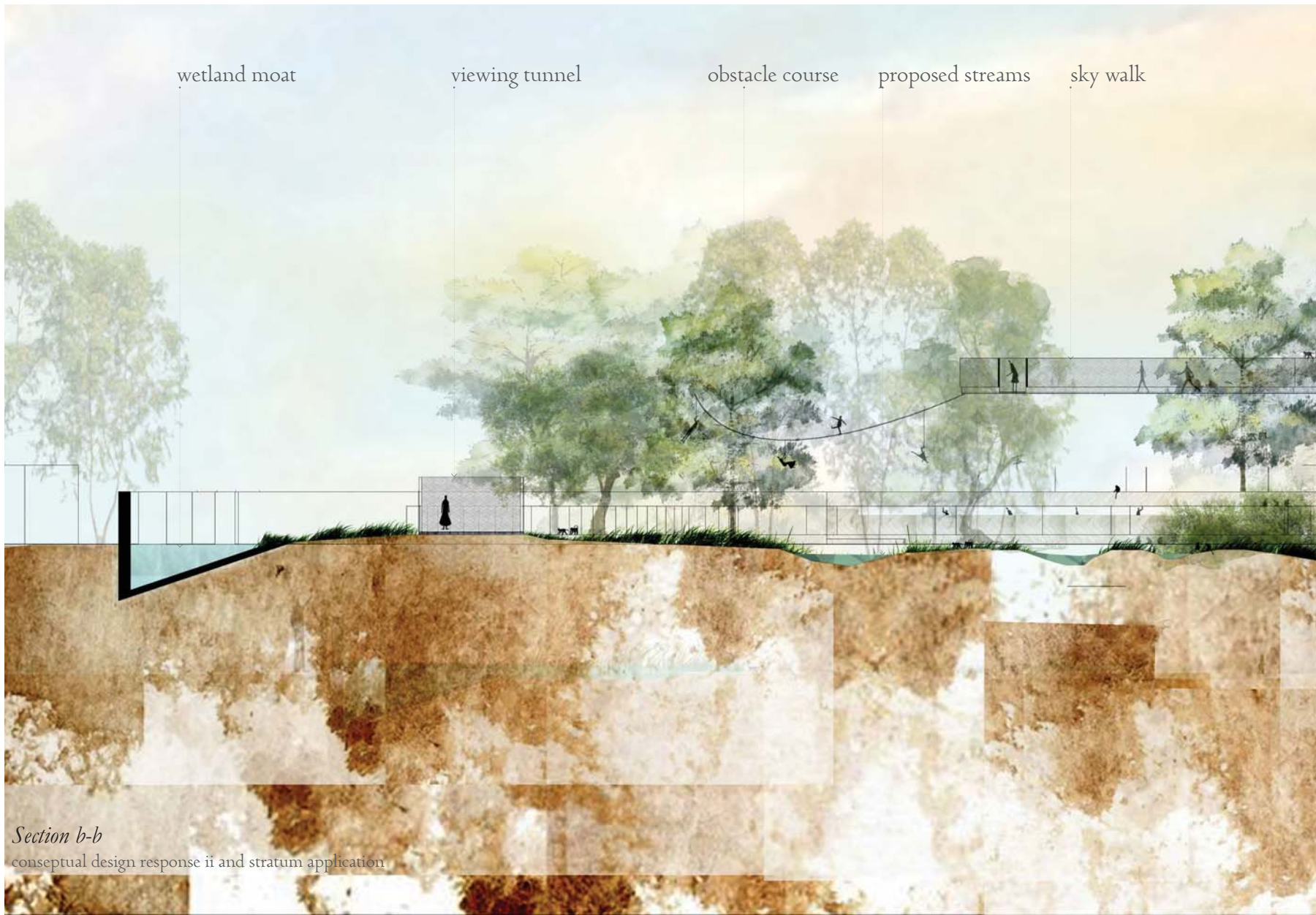
V_55. Sectional elevation b-b: Draft design response to stratum concept application showing moat barrier, and skywalk (Author 2014).
