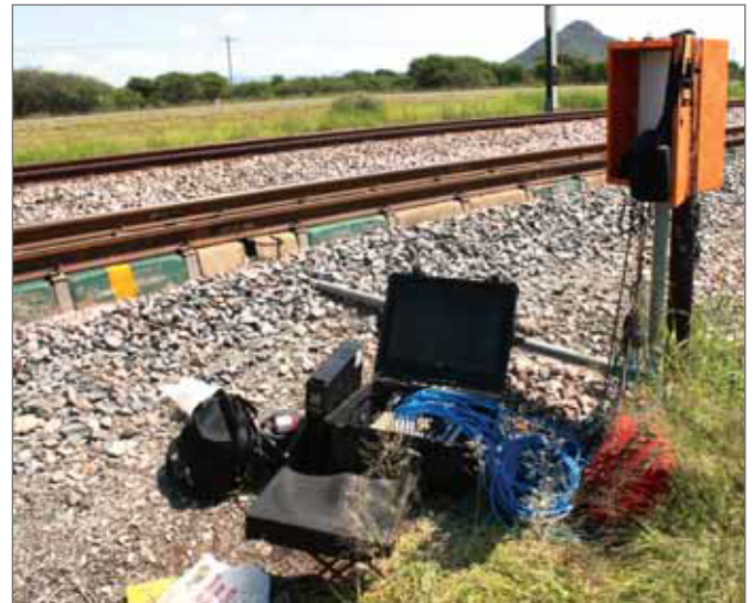
Figure 3: Multi-Depth Deflectometer connectors coupled to the logging equipment on site
