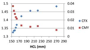
**Figure 8** Variation of  $C_{Fx}$  (left ordinates) and  $C_{My}$  (right ordinates) with different HCL for  $\alpha = 90^{\circ}$  and  $\beta = 0^{\circ}$
