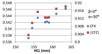
**Figure 9** Variation of  $C_{Fx}$  (left ordinates) and  $|C_{Fz}|$  (right ordinates) with different HCL for  $\alpha = 30^{\circ}$  and  $\beta = 0^{\circ}$
