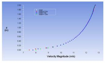
Figure 5 Mean velocity profile at x=0 (inlet), 0.5, 1 and 1.5 m
