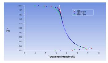
**Figure 6** Turbulence intensity profile at x=0 (inlet), 0.5, 1 and 1.5 m
