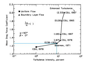
Figure 7 Drag coefficient measured for the case  $\alpha = 90^{\circ}$ and  $\beta = 0^{\circ}$  in several studies [3]
