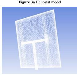
Figure 3b Heliostat mesh
