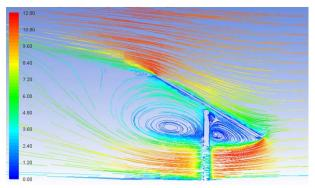
Figure 13 Streamlines coloured by velocity magnitude (m/s) in z-x plane around inclined heliostat (b), HCL=153.5 mm
