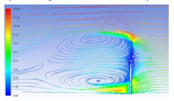
Figure 14 Streamlines coloured by velocity magnitude (m/s) in z-x plane around vertical heliostat, HCL=270 mm
