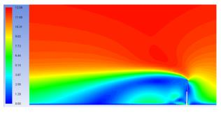
Figure 11 Velocity (m/s) flow field in z-x plane around vertical heliostat, HCL=163.5 mm
