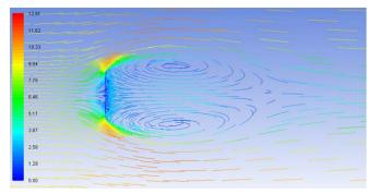
**Figure 15** Streamlines coloured by velocity magnitude (m/s) in x-y plane for a vertical heliostat, HCL=153.5 mm
