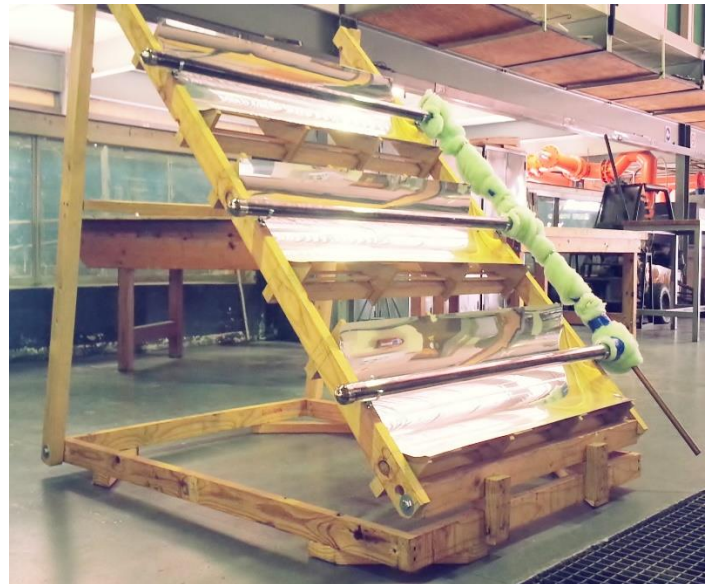
Figure 1 Photograph of evacuated tubes arrangement.
